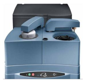
Differential Scanning Calorimetry or DSC is a thermal analytical method for performing heat analysis; measures the amount of energy absorbed while the sample is being heated, cooled, or held at a constant temperature. DSC is following the same principle of measurement as DTA. The main application areas of DSC are studies on phase changes such as exothermic and endothermic decomposition. DSC is used to measure thermal changes such as specific heat
